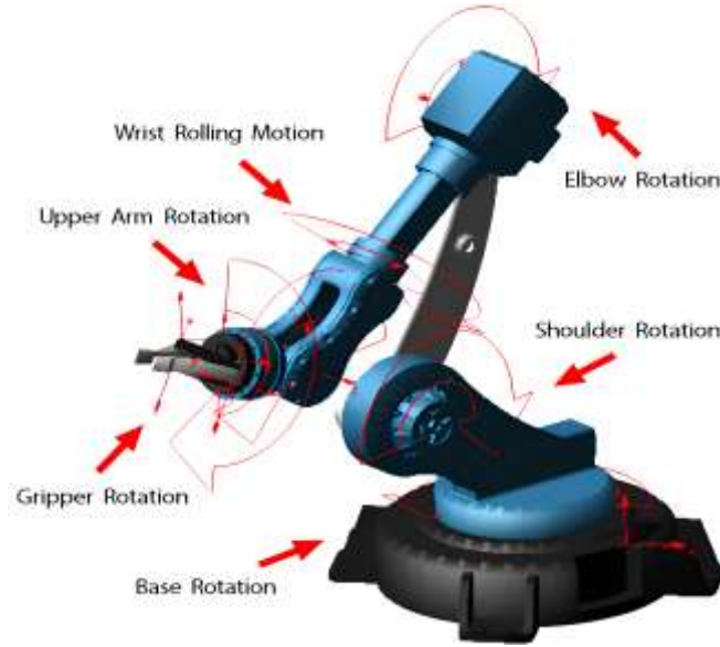
Figure 1. Structure of a Six-Degree-of-Freedom Robotic Arm with Rotational Constraints.
