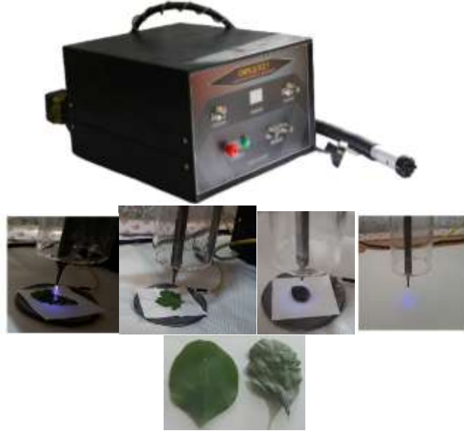
Figure 3. The fabricated laboratory prototype (top), the produced pulsed plasma (middle), plant sample before (bottom left), and plant after 10 min of plasma application (bottom right).
