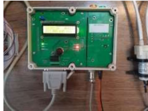
Figure 5. Data logging process from the olfactory sensors using the designed Arduino board.
