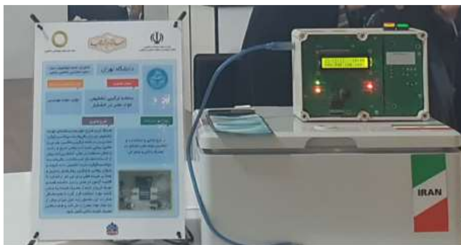
Figure 2. A complete view of the constructed hybrid system (electronic nose + machine vision) as displayed at the research exhibition.
