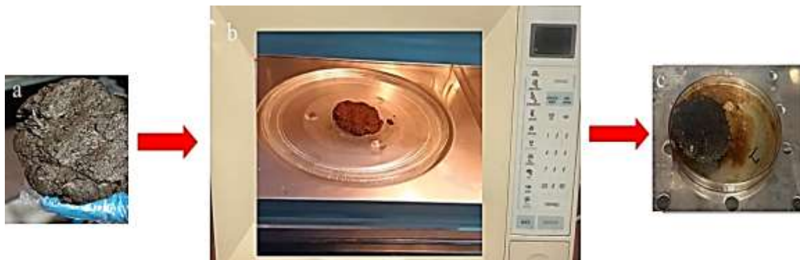
Figure 1. The process of microwave sludge drying: a) dewatered sludge, b) microwave process for drying, c) dried sludge by microwave
