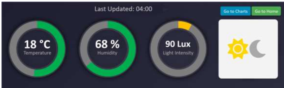
Figure 9. Graphical interface status at 04:00 on July 2, 2025, showing normal temperature and relative humidity conditions and a warning status for light intensity due to the scheduled shutdown of the artificial lighting system.
