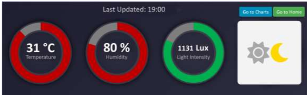
Figure 10. Graphical interface status at 19:00 on July 2, 2025, showing warning conditions for temperature and relative humidity immediately after power restoration.
