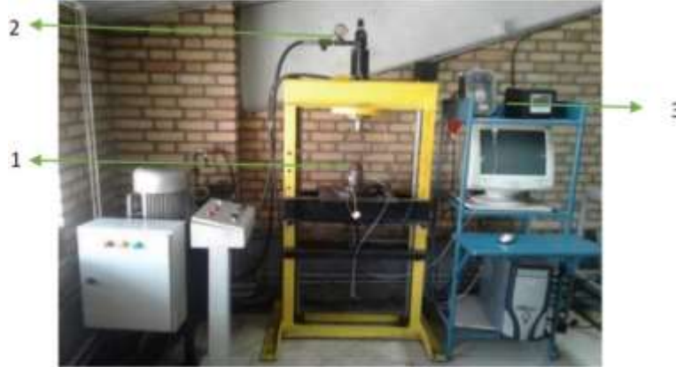
Figure 2. Press machine with pellet die: 1) Die and position, 2) Pressure gauge and flow control valve, 3) Thermocouple and controller
