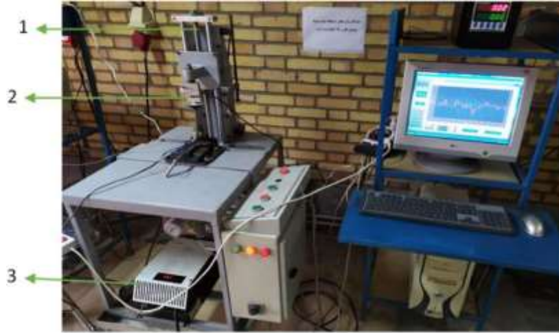
Figure 4. Biological Material Test (B.M.T) machine (Instron): 1) Ball screw for moving the load cell at a specified speed, 2) Load cell, and 3) Inverter
