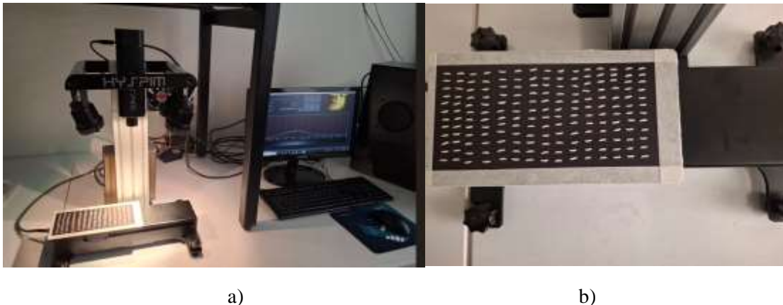
Figure 2. a) Hyperspectral imaging system; b) Arrangement of rice grains on the scanner.
