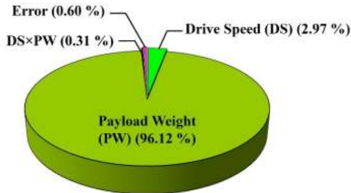
Figure 2. Contribution percentage of causative variables to the slippage of the unmanned tracked vehicle
