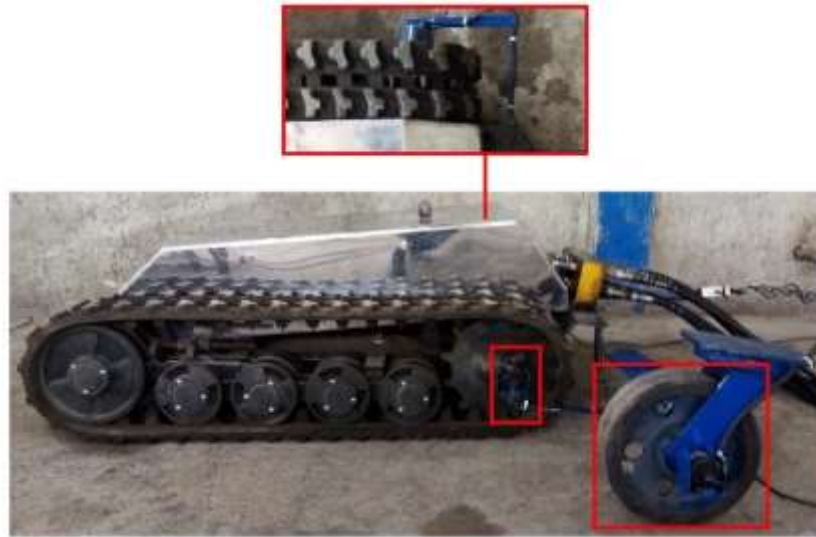
Figure 1. The unmanned tracked vehicle outfitted with three encoder transducers (right and left driving tracks, and auxiliary rigid wheel)
