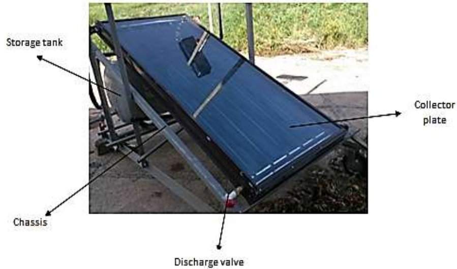
Figure 1. Flat plate solar collector model, Solar Polar Company, IRAN.
