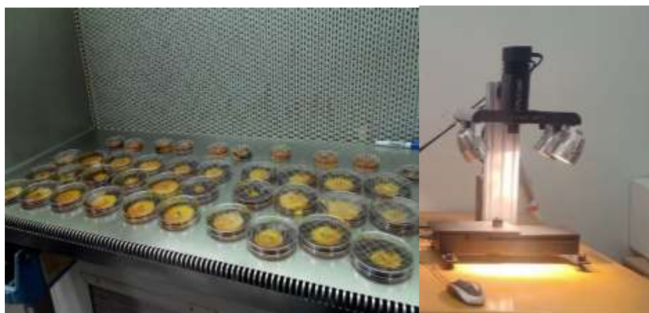
Figure 1. The studied fungal isolates (left) and the used hyperspectral imaging system (right).
