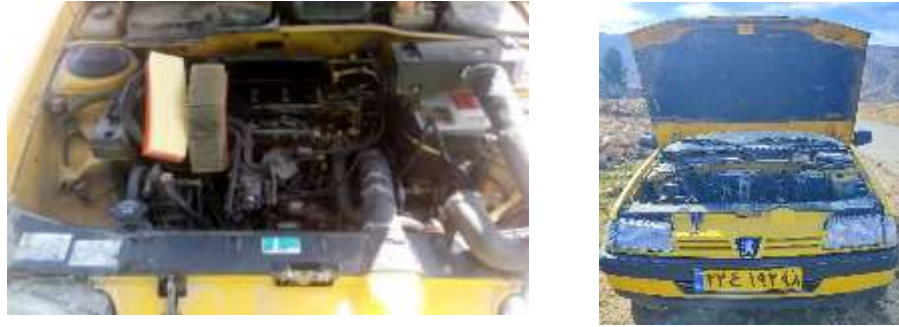
Figure 4. XU7 engine used in testing.
