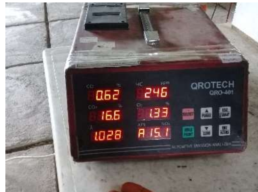
Figure 5. Five-gas test device connected to the catalystr.
