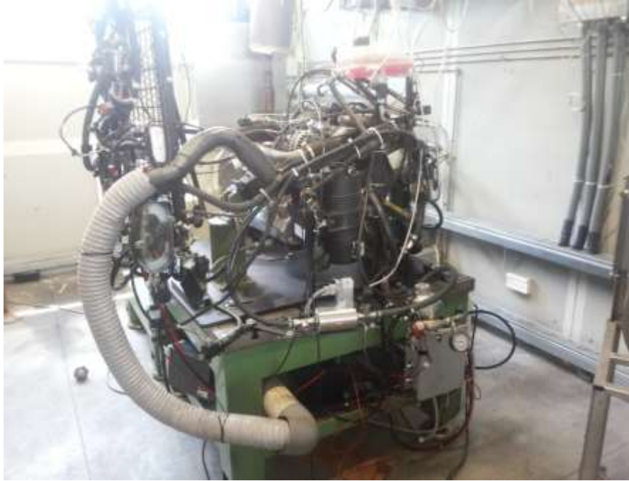
Figure 2. The PIAGGIO four-cylinder petrol engine and the dynamometer in a standard test room
