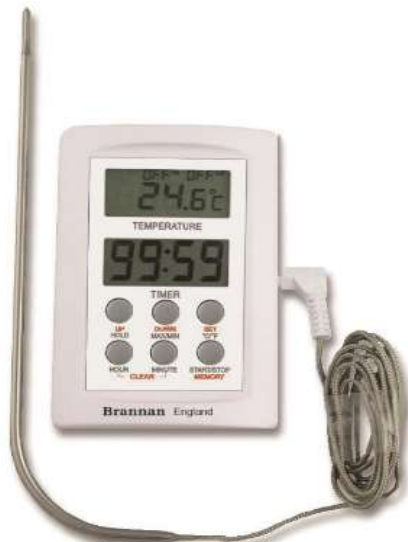
Figure 3. Thermometer used for measuring the temperature of the exhaust gas emissions
