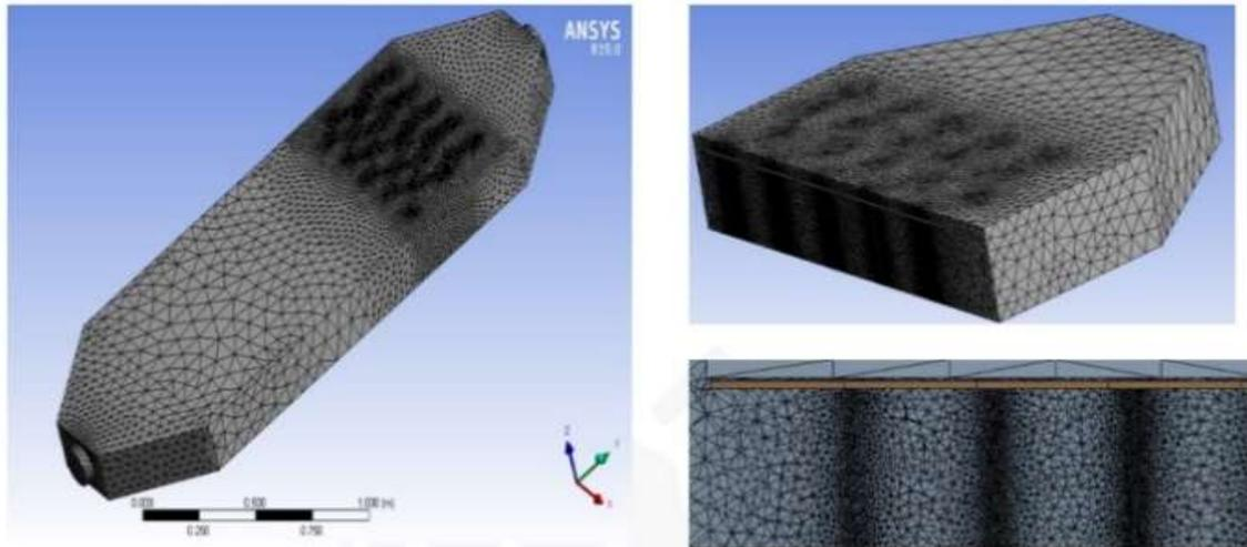
**Figure 4.** Meshed Model of the Solar Collector.
