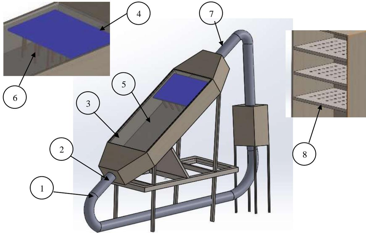
**Figure 2.** Schematic diagram of solar dryer system: 1) Collector inlet, 2) Fan, 3) Glass cover, 4) PV panel, 5) Absorber plate, 6) Copper pipes containing paraffin, 7) Collector outlet, 8) Sample tray location.
