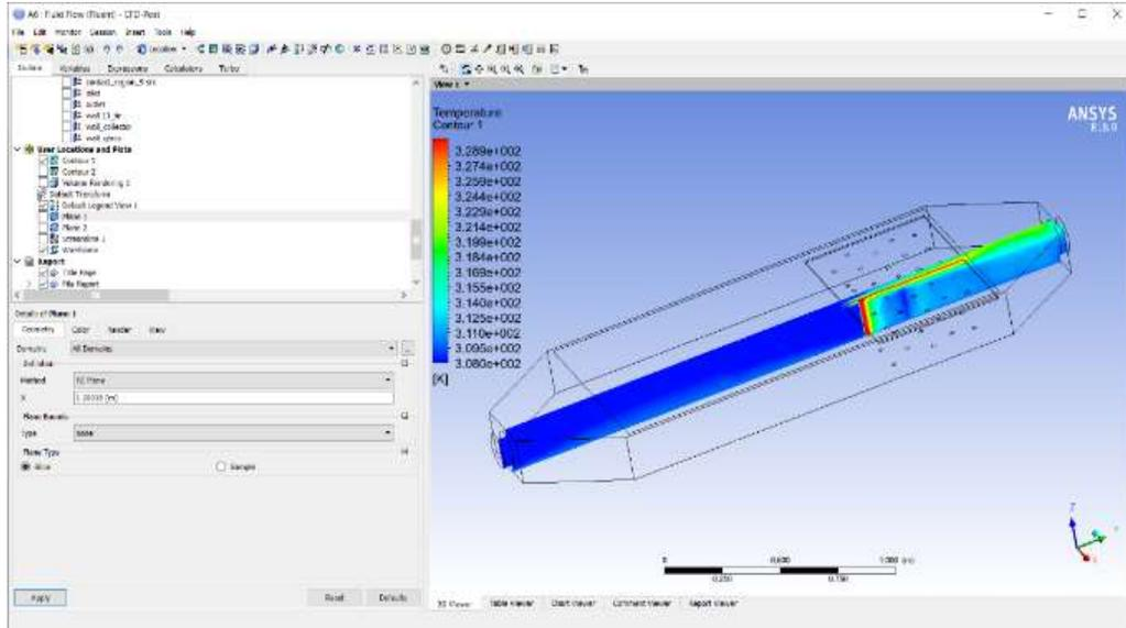
**Figure 8.** Thermal distribution contours in the collector during the discharge process of the PCM.
