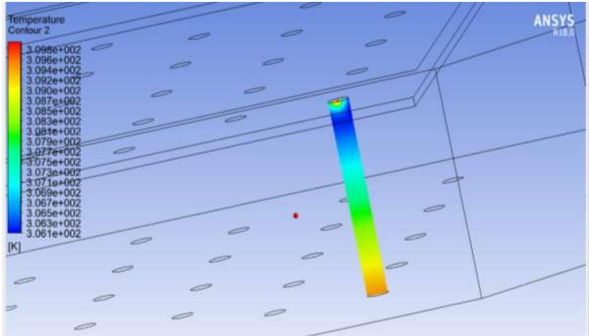
**Figure 6 .** Thermal contours for the paraffin-containing pipe during heat absorption by the PCM.
