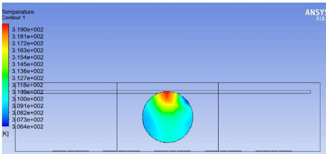
**Figure 9.** Thermal contours of the collector outlet during the discharge process of the PCM.
