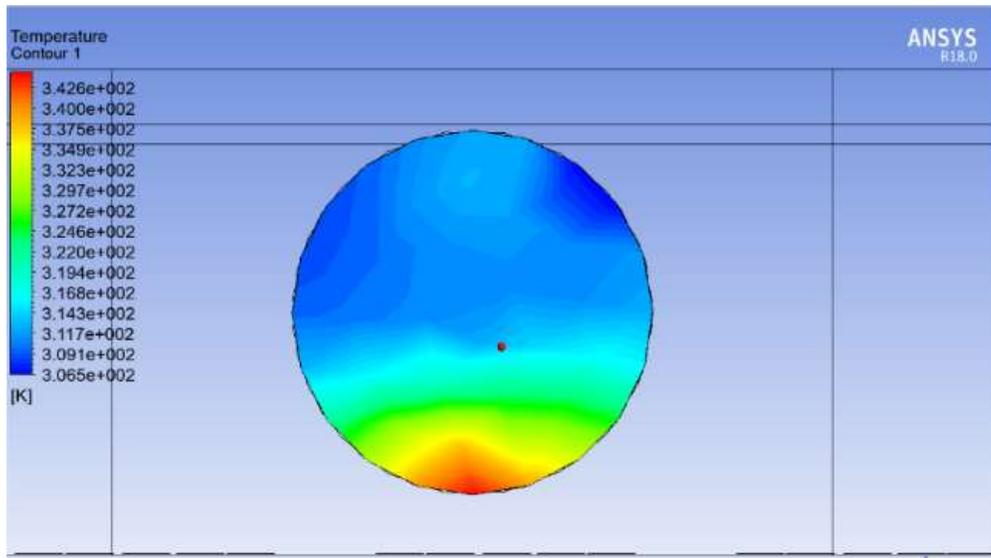
**Figure 7.** Thermal contours of the collector outlet during heat absorption by the PCM.
