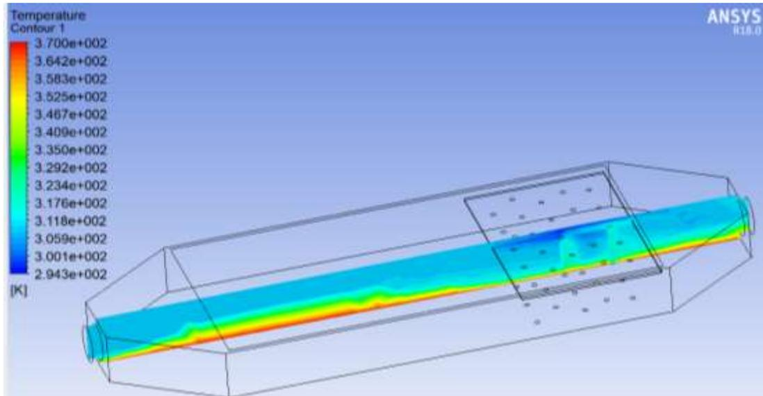
**Figure 5.** Thermal Contours for the Flat-Plate Solar Collector during the Heat Absorption by the PCM.
