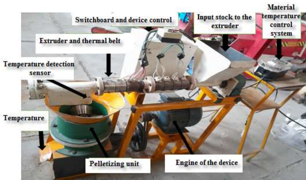
Figure 4. Pellet making machine for pistachio green shell
