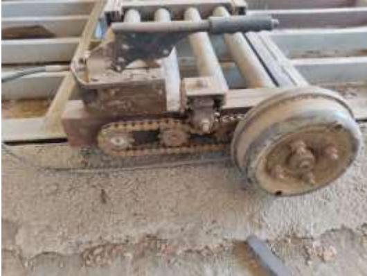
Figure 4. Drum-brake system on chassis dynamometer
