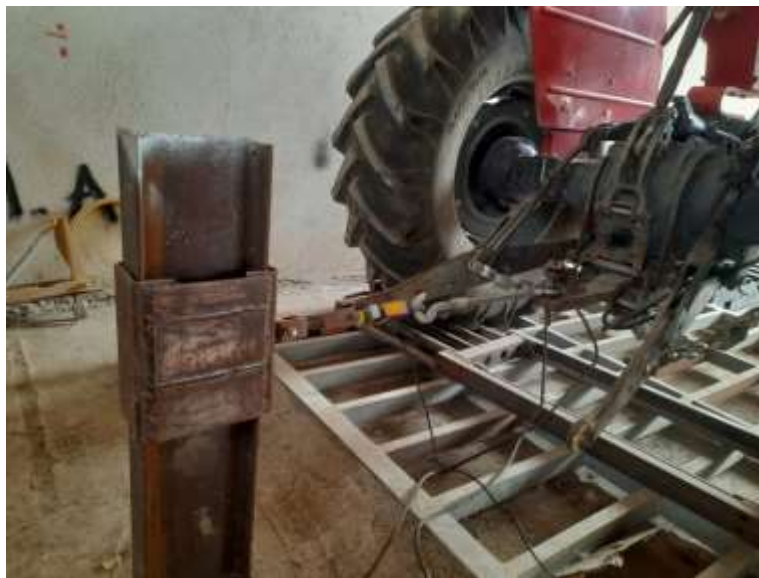
Figure 7. Placing the tractor on the dynamometer during dynamometer performance evaluation tests
