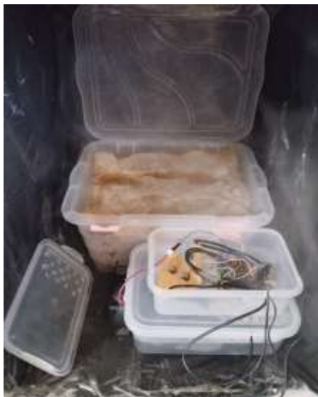
Figure 3. Mushroom growth chamber with humidity control circuit
