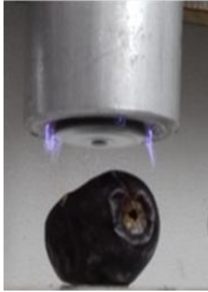
Figure 2. The sample plasma treatment by the sliding rotary arc reactor
