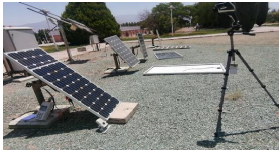
Fig 1. The details of taking a thermal image of the panel
