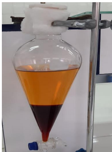
Fig 2. Separation of glycerol from biodiesel
