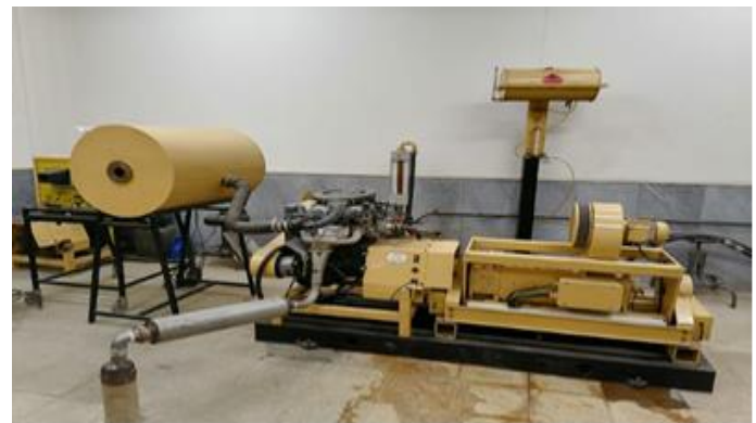
Fig 1. Engine set up and dynamometer coupled to it
